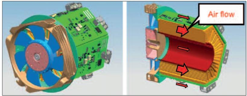
this configuration, the whole DC link of the inverter is integrated into the housing. A further advantage is the thermal decoupling of the capacitor from the heat sink and the PCBs. The ring shaped capacitor can be realized by a simple winding process and is already established for automotive applications.
