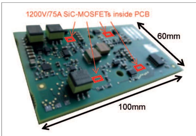
Figure 3: PCB-based half bridge with four embedded SiC MOSFETs and integrated functions
