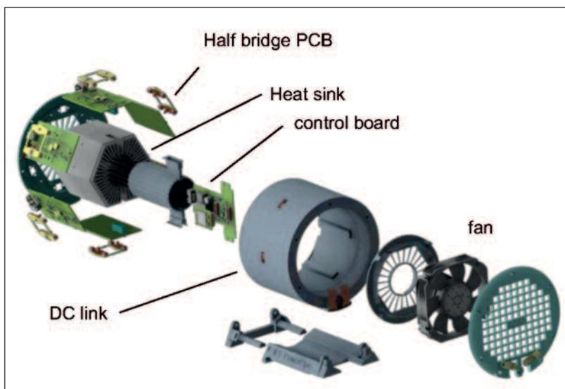
DC link capacitance in form of a snubber capacitor (CeraLink™). Furthermore, on each PCB a temperature sensor is placed near to the hottest spot.
