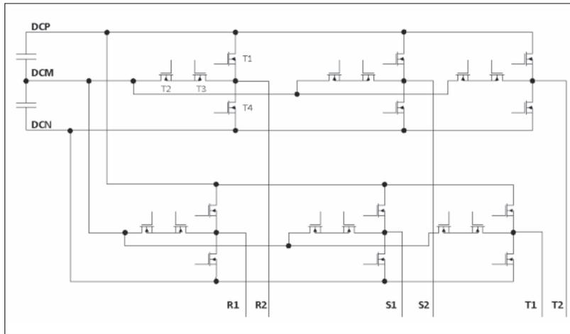
Figure 2: Dual T-type topology with SiC MOSFETs
