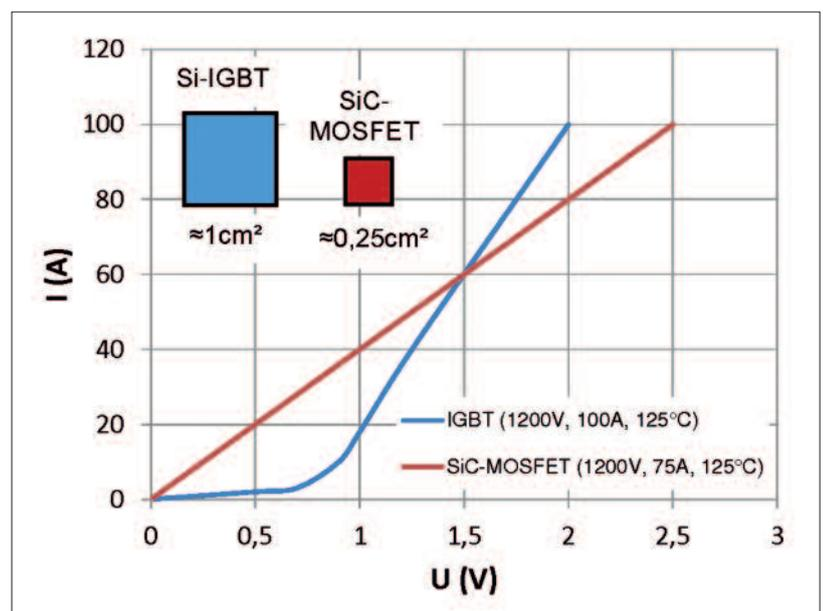
Figure 1: Output characteristics of IGBT and SiC MOSFET and comparison of chip area
