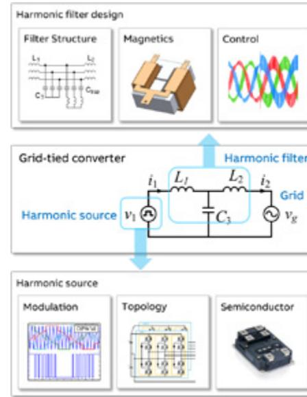
Fig. 1: Power electronic system hierarchy
