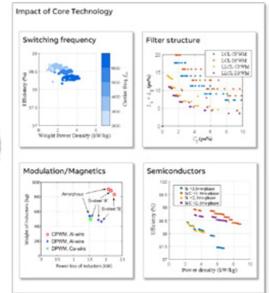
Fig. 2: Core technology breakdown and impact on grid-tied converter
