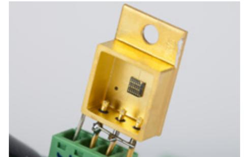
Fig. 2: Diamond power diodes on monocrystalline diamond substrates
