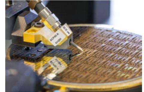
Fig. 1: AlScN/GaN wafers for on-wafer characterization
