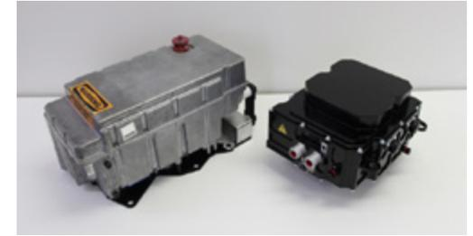
Fig. 1: Two power train inverters (left: Si IGBT based 200kW inverter, right: SiC MOSFET based 220kW inverter)
