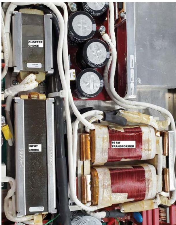
**FIG 4** 10 kW transformer, input choke, and chopper choke.
