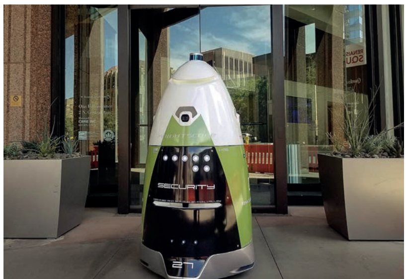
Knightscope's mobile robots are completely autonomous, using a system of LIDAR, GPS, sonar, IMUs, 4K cameras and high-fidelity audio. The robot has five sensor types—similar to humans but with far greater acuity.
