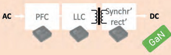
➤ Figure 3. Typical GaN-based power supply with analogue control.
