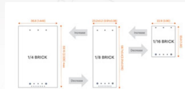
*Fractional bricks are a range of power modules with de facto industry-standard sizes and footprints.*
