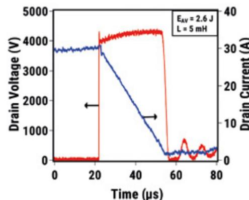
Figure 6: Drain-current and drain-voltage waveforms from UIS measurement performed on a 3.3-kV SiC MOSFET with monolithically integrated MPS diode
