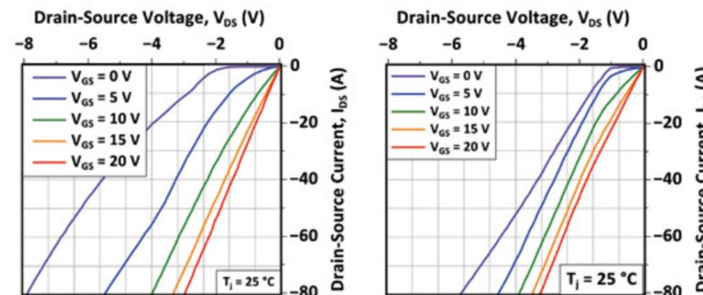
Figure 3: Third-quadrant I-V characteristics measured on 3.3-kV, 40-mΩ, discrete SiC MOSFET (left) and SiC MOSFET with monolithically integrated MPS diode (right)
