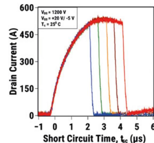
Figure 7: Drain-current waveform recorded during a short-circuit test performed on a 3,300-V SiC MOSFET with monolithically integrated MPS diode at a DC-link voltage of 1,200 V
