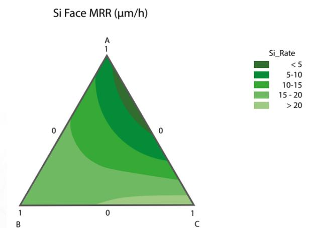
Figure 2: Representative silicon face MRR ( $\mu\text{m}/\text{hour}$ ) response surface in a three-component mixture design using 3- $\mu\text{m}$  monocrystalline diamond (Source: Pureon)
