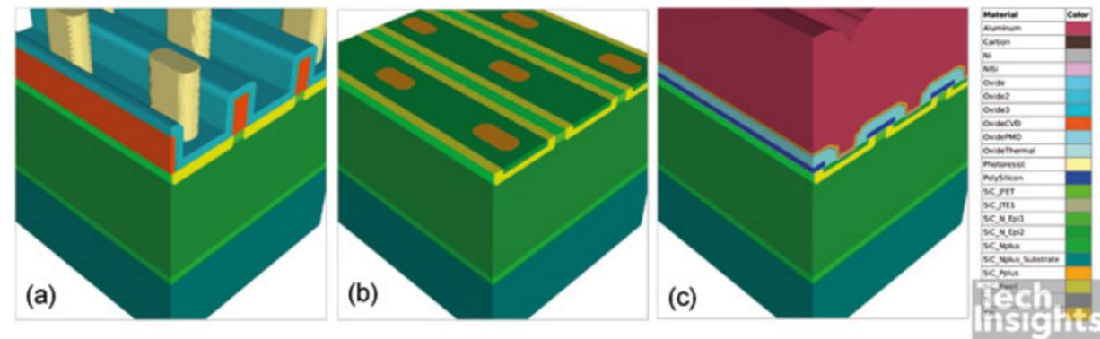
Figure 3: Selected 3D emulation results at various stages of the STMicorelectronics SCT040H65G3AG flow — (a) right after P+ blocking lithography; (b) at the completion of P+ implant module; (c) just after top metal deposition
