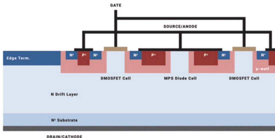
Figure 4: Cross-sectional device schematic of 3.3-kV SiC MOSFET with monolithically integrated Schottky rectifier
