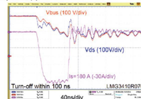
Figure 7: Short-circuit protection with the LMG341x parts showing a fast turn-off response (Source: Texas Instruments)
