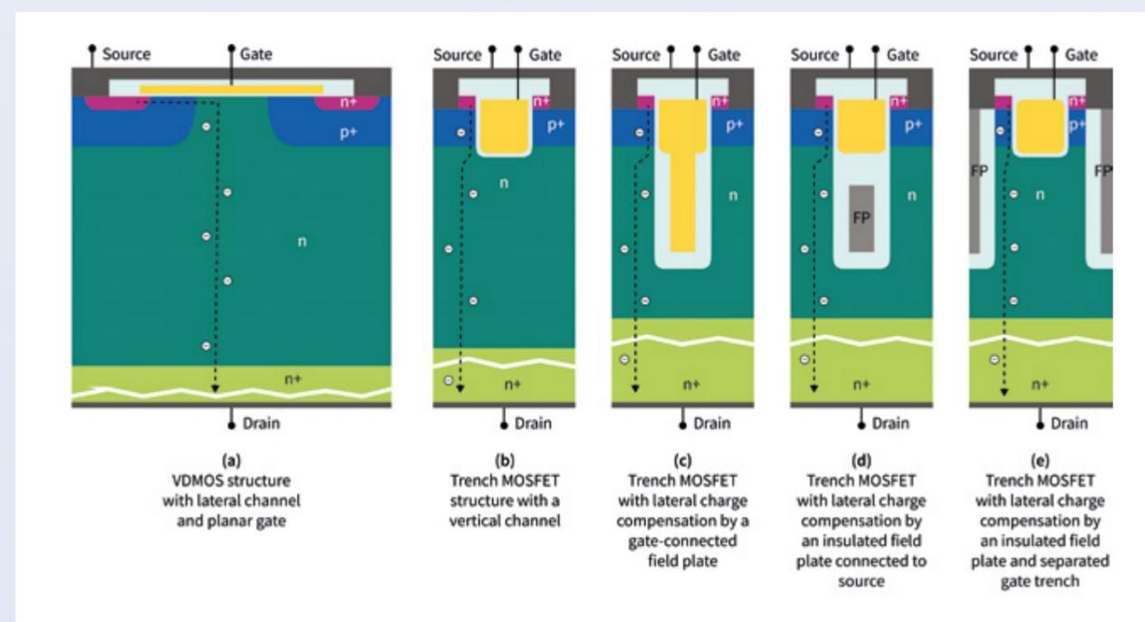
Figure 1: Exemplary device structures depicting the evolution of a power MOSFET
