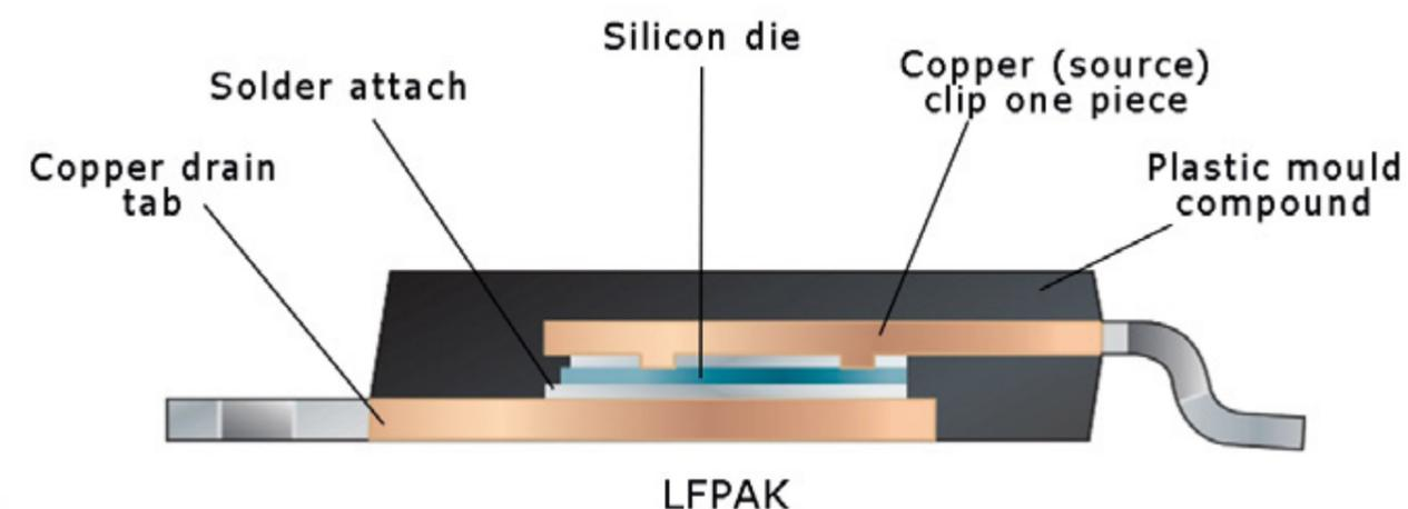
Figure 1: LFPAK internal structure (Source: Nexperia)
