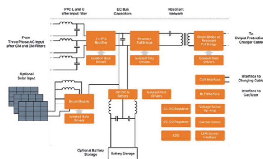
Figure 2: EV charging station block diagram (Source: onsemi)
