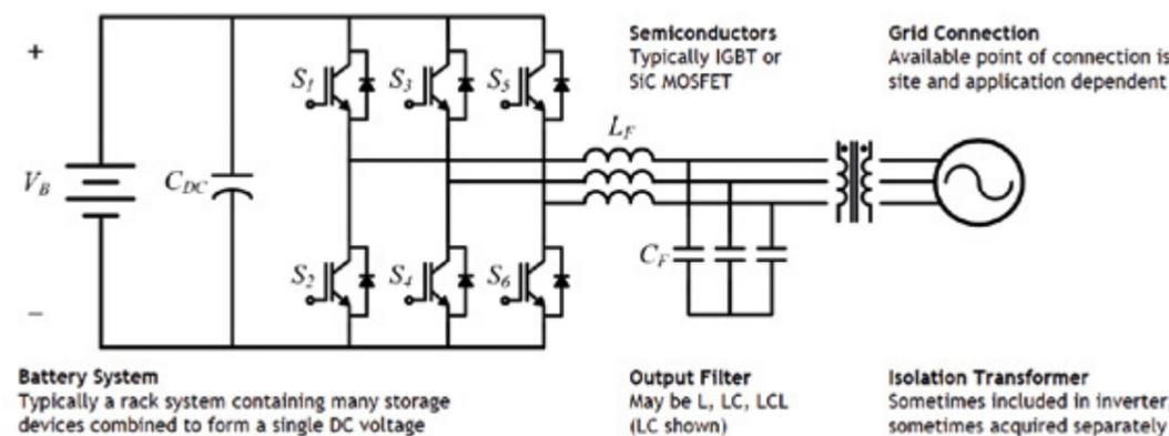
Figure 6: Conventional single-stage PCS<sup>1</sup> (Source: Muller)
