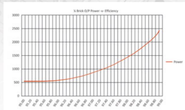
The effect of incremental efficiency improvements unlocks more power as overall efficiency increases.
