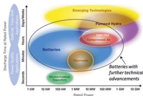
Figure 1: Energy storage techniques versus power and discharge time (Source: U.S. Department of Energy, "Potential Benefits of High-Power, High-Capacity Batteries," January 2020)
