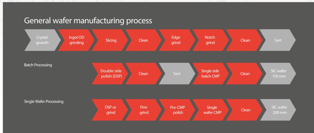
Figure 1: Manufacturing SiC wafers (Source: Pureon)
