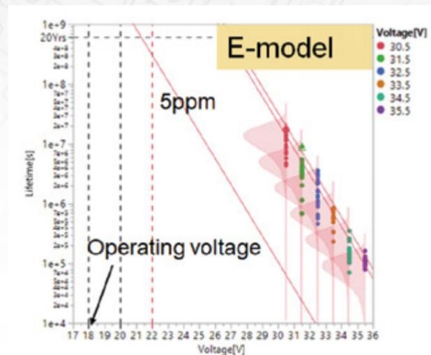
Figure 3:  $V_{GS}$  against lifetime performance at  $V_{GS}$  much higher than used in real-world applications (Source: onsemi)
