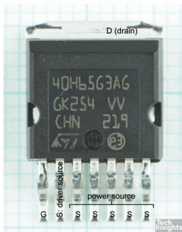
Figure 1: STMicorelectronics' SCT040H65G3AG in a seven-lead H2PAK package
