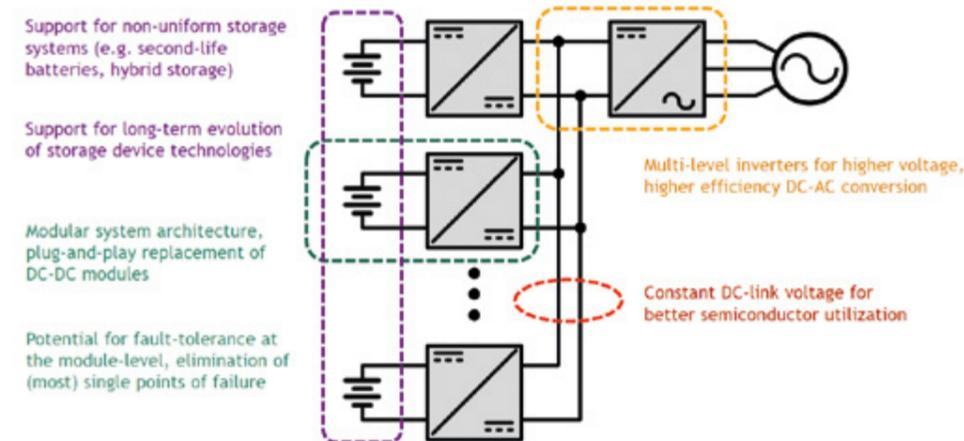
Figure 7: Multi-stage PCS<sup>1</sup> (Source: Muller)
