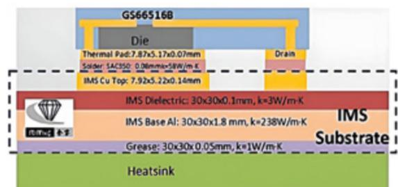
Thermal conduction path of each transistor
