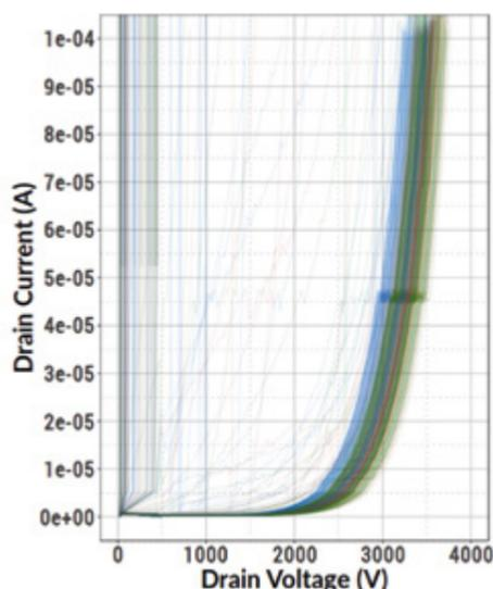
Figure 5: Third-quadrant breakdown characteristic measured on 3.3-kV SiC MOSFETs with monolithically integrated MPS diodes
