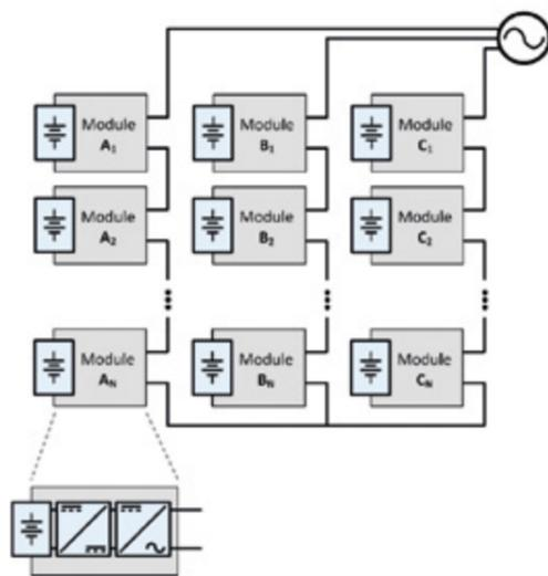
Figure 9: A cascaded, series-connected PCS<sup>1</sup> (Source: Muller)
