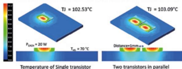
Thermal finite element analysis simulation results of GaN HEMTs on the IMS substrate (Source: IEEE)
