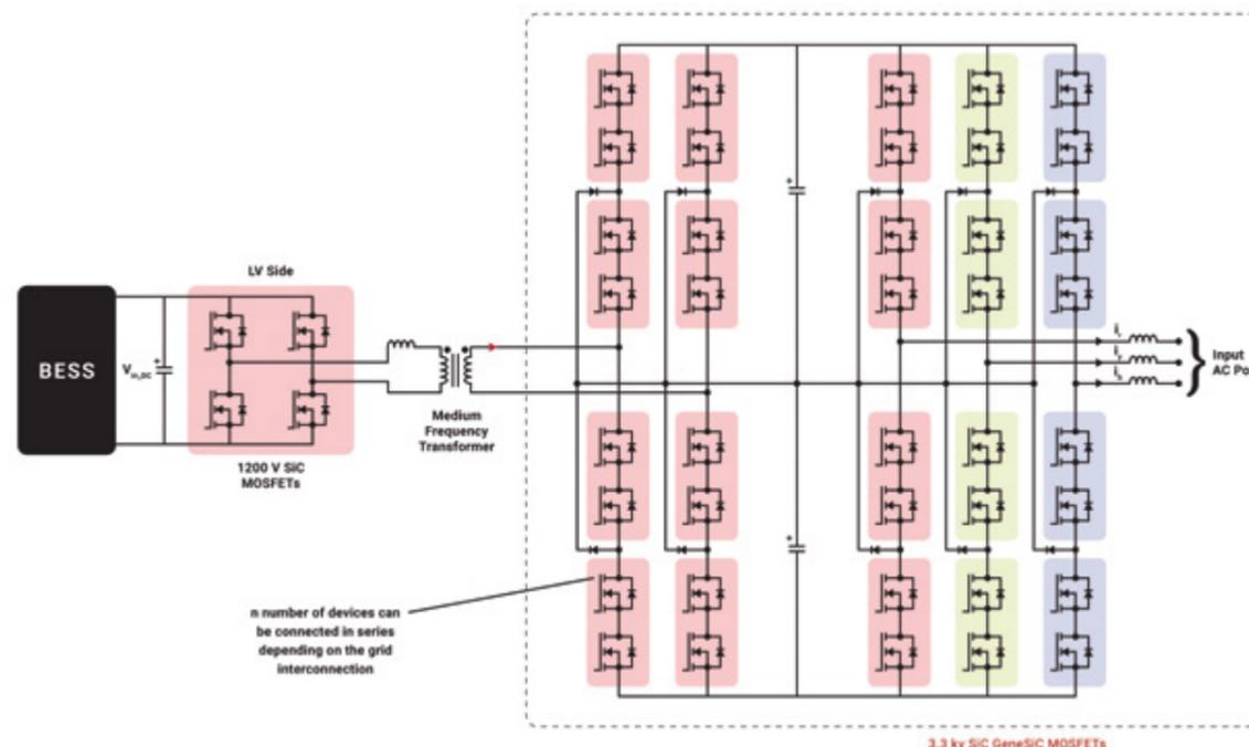
Figure 2: System topology for interconnecting the BESS system to an MV grid
