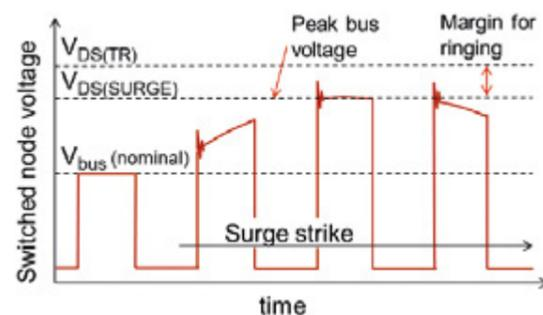
Figure 6(a):  $V_{DS(SURGE)}$  and  $V_{DS(TR)}$  datasheet specifications for TI's GaN devices (Source: Texas Instruments)
