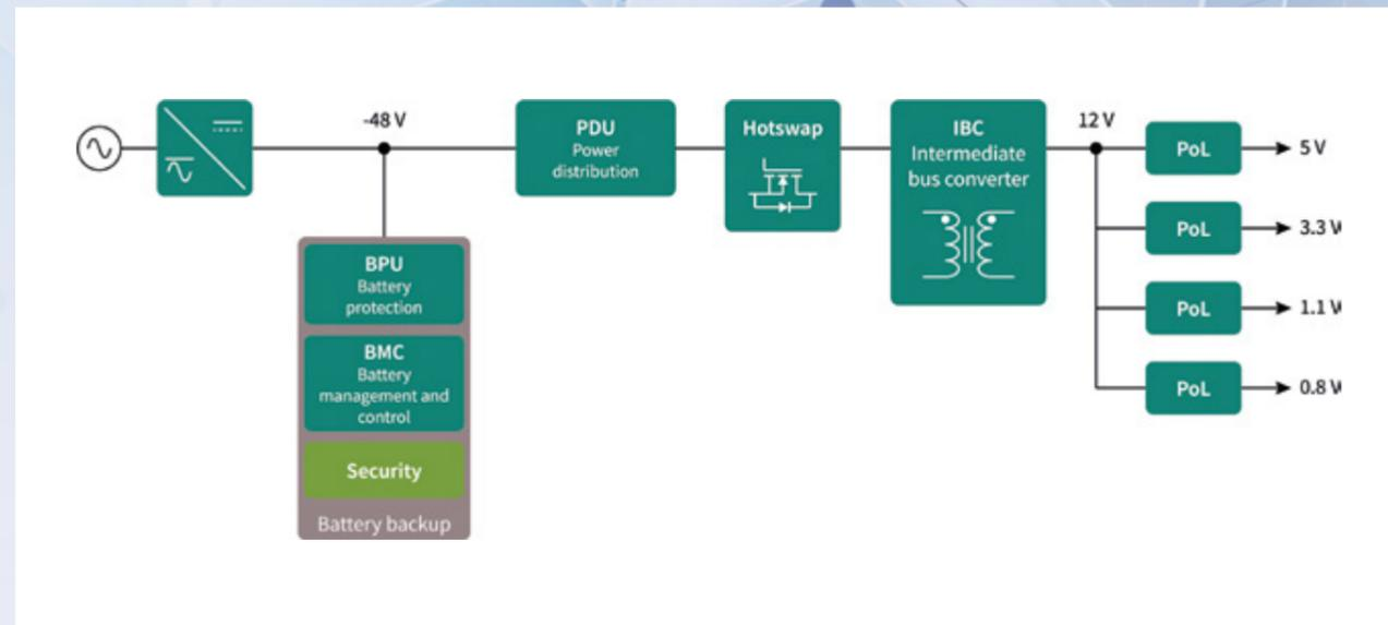
Figure 3: System diagram of the IBA
