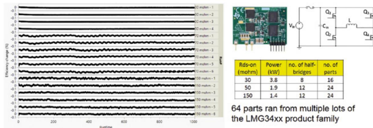
Reliable in-system operation for both hard and soft switching: stable running with efficiency within 0.1%
