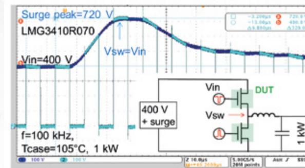
Figure 6(b): Surge waveforms for the LMG3410R070 device showing switching (light blue curve) operation during the  $V_{IN}$  (dark blue) surging to 720 V (Source: Texas Instruments)
