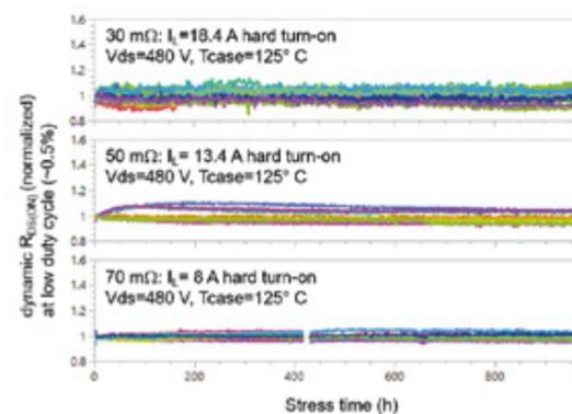
Figure 3: GaN charge trapping mechanism and dynamic  $R_{DS(on)}$  measurements from TI (Source: Texas Instruments)
