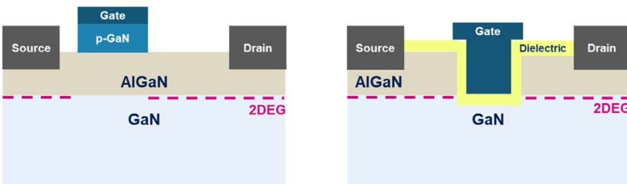
Figure 2: E-mode (normally off) HEMT realizations: p-gate (left) and recessed gate (right) (Source: STMicroelectronics)
