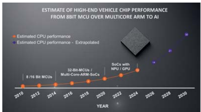
Figure 2: Performance increase of car semiconductors over the last year. The estimation is based on the semiconductor types used during evaluated time frame and is normalized to the performance of 2010. By 2024 the performance increased by about 10x. This trend will keep accelerating.
