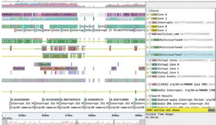
Figure 4: Snapshot of the Green Hills Software History viewer, displaying a recording of a system runs on a multicore processor, integrates multiple OSES, and executes mixed-criticality functions.
